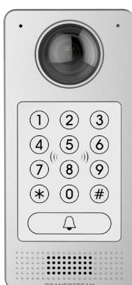
You can integrate IP Video Door Stations, like our GDS3710, with the UCM series. This allows you to use your endpoints to track, monitor and control access to any building.
