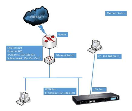
Figure 10: UCM6510 Network Interface Method: Switch
