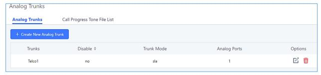
Figure 117: Analog Trunk with SLA Mode Enabled
