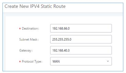
Figure 18: UCM6510 Static Route Configuration
