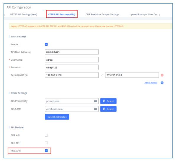
Figure 269: Enable PMSAPI
