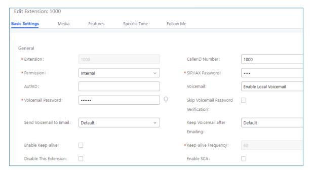
Figure 241: Enabling SCA Option under Extension's settings
