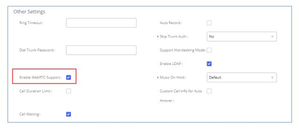
Figure 155: Enabling WebRTC on extensions
