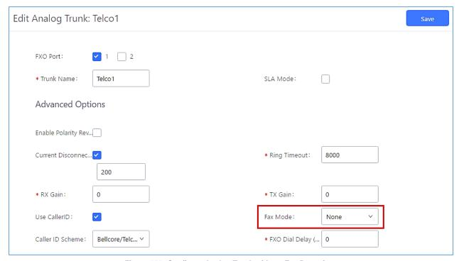
Figure 209: Configure Analog Trunk without Fax Detection
