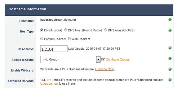
Figure 23: Register Domain Name on noip.com
