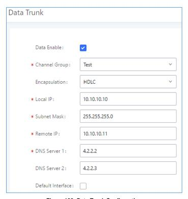
Figure 108: Data Trunk Configuration
