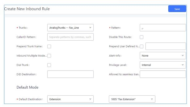
Figure 212: Configure Inbound Rule for Fax
