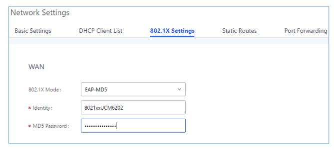
Figure 16: UCM6510 using 802.1X EAP-MD5
