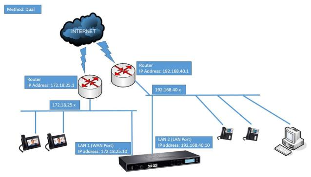
Figure 11: UCM6510 Network Interface Method: Dual
