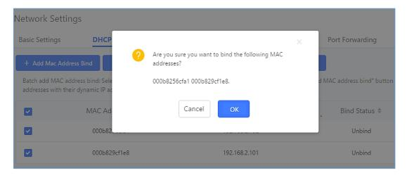
Figure 14: Batch Add MAC Address Bind
