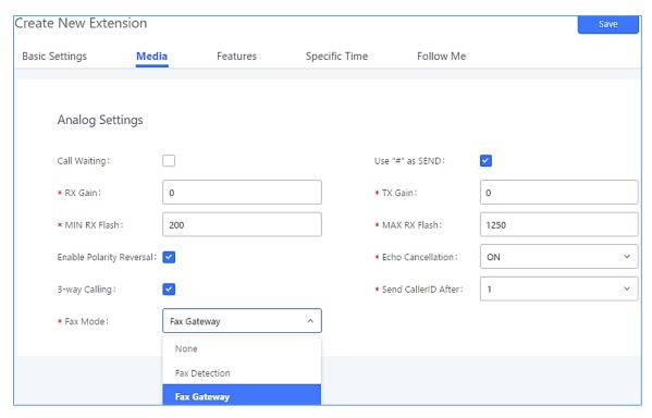
Figure 211: Configure Extension for Fax Machine: Analog Settings
