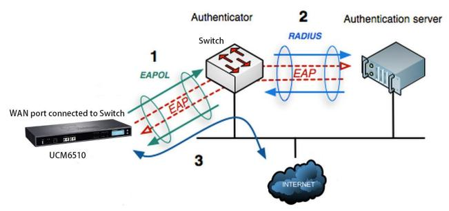
Figure 15: UCM6510 using 802.1X as Client
