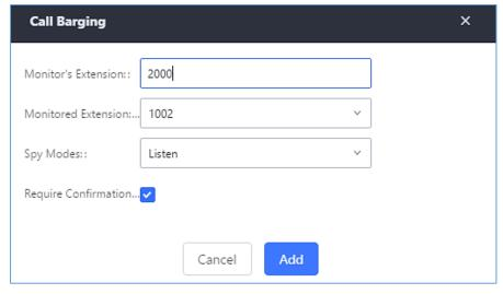
Figure 235: Configure to Monitor an Active Call
