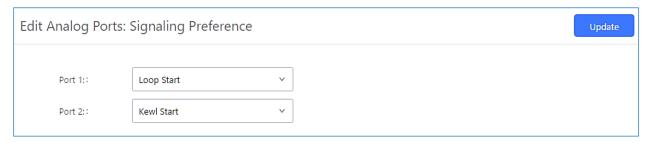
Figure 102: FXS Ports Signaling Preference
