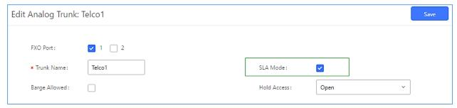
Figure 116: Enable SLA Mode for Analog Trunk
