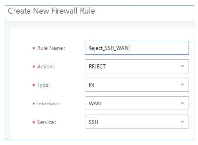
Figure 26: Create New Firewall Rule
