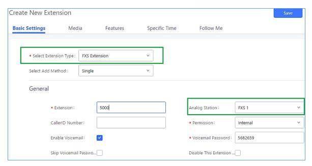
Figure 210: Configure Extension For Fax Machine
