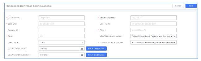
Figure 41: LDAP Client Configurations
