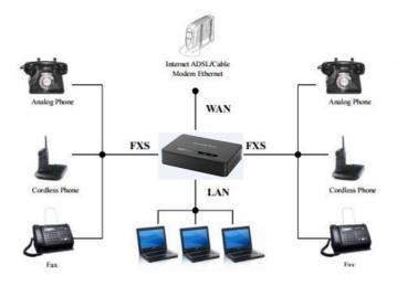
Figure 3: Connecting the HT818
