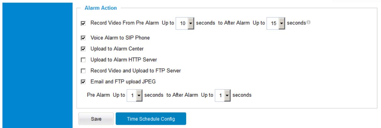
Figure 24-2: Motion Detection Configuration Page
