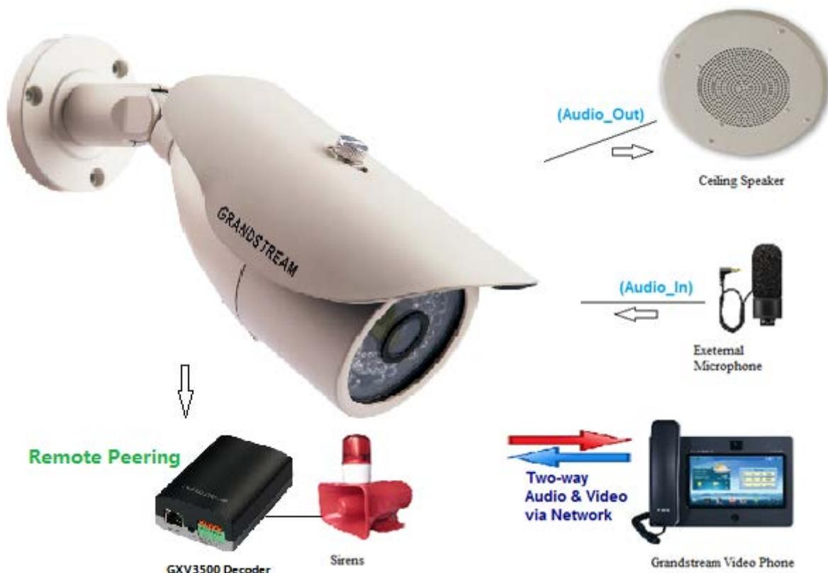
**Figure 6: Application Peripheral Connection for GXV3672\_HD/FHD v2**
