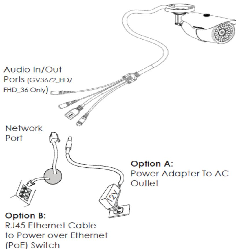
**NOTE:** Choose Option A if using the power supply; or choose Option B if using a Power over Ethernet (PoE) switch.
