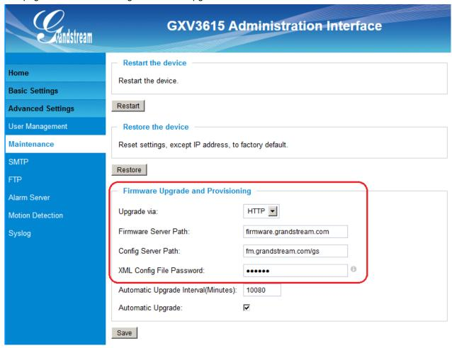
Figure 18: Firmware Upgrade and Provisioning
