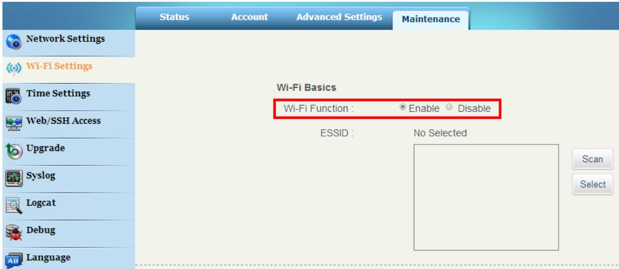
Figure 3: Turn On/Off Wi-Fi from Web UI
