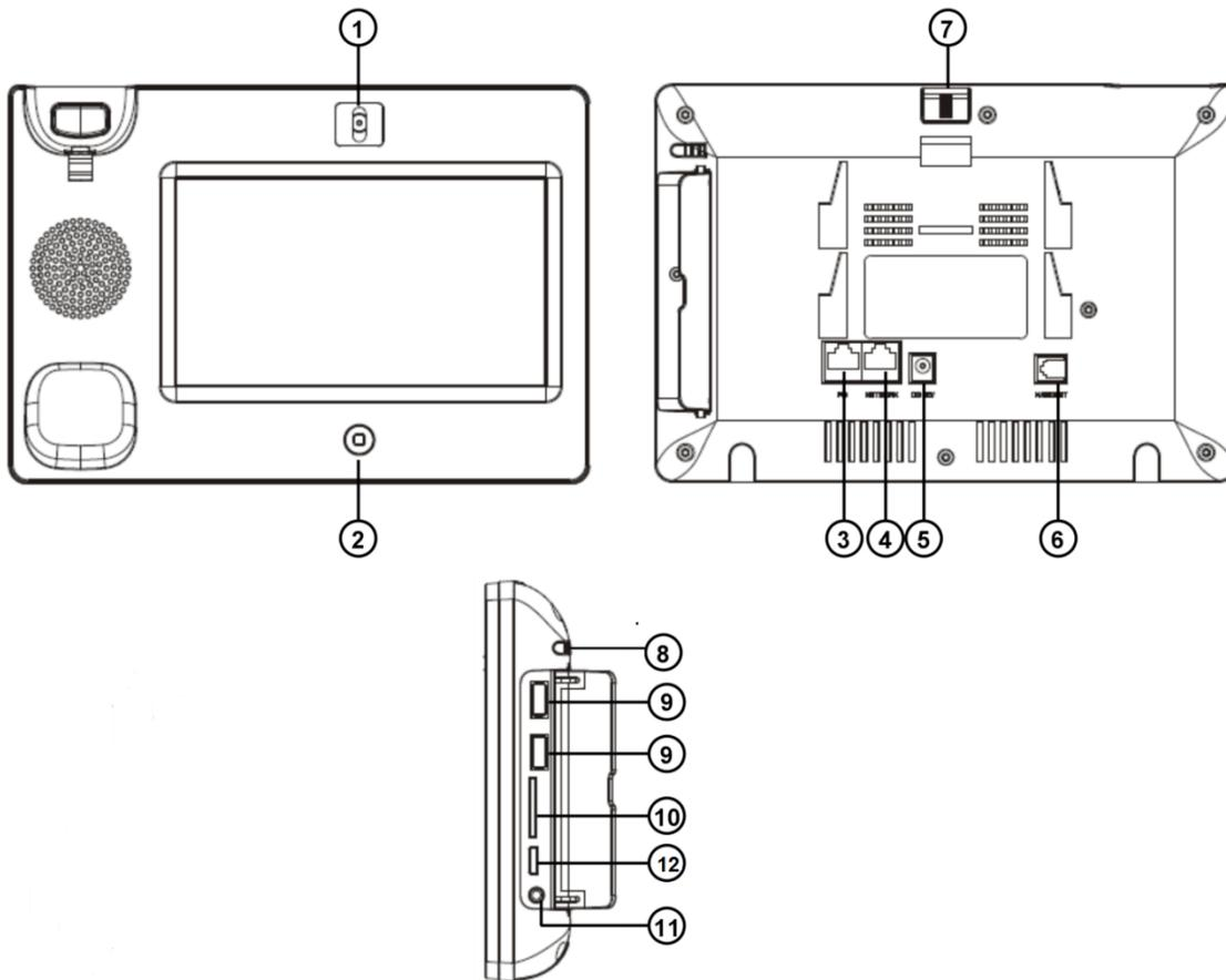
Figure 2: GXV3175V2 Ports and Interface
