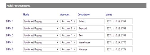
Figure 7: Sending Multicast Page Configuration by using MPK
