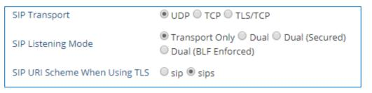
Figure 6 : Configure TLS as SIP Transport
