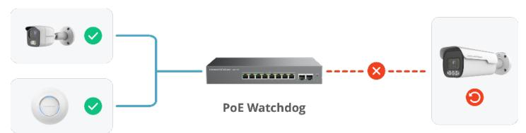
**Anomaly Detection:** The PoE switch continuously monitors the network operation status of connected powered devices (such as cameras, APs, IP phones, etc.).
