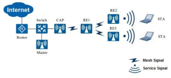
Figure 6: Mesh Network Use Case
