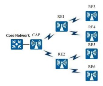
Figure 4: Mesh Network - Hierarchical Mode
