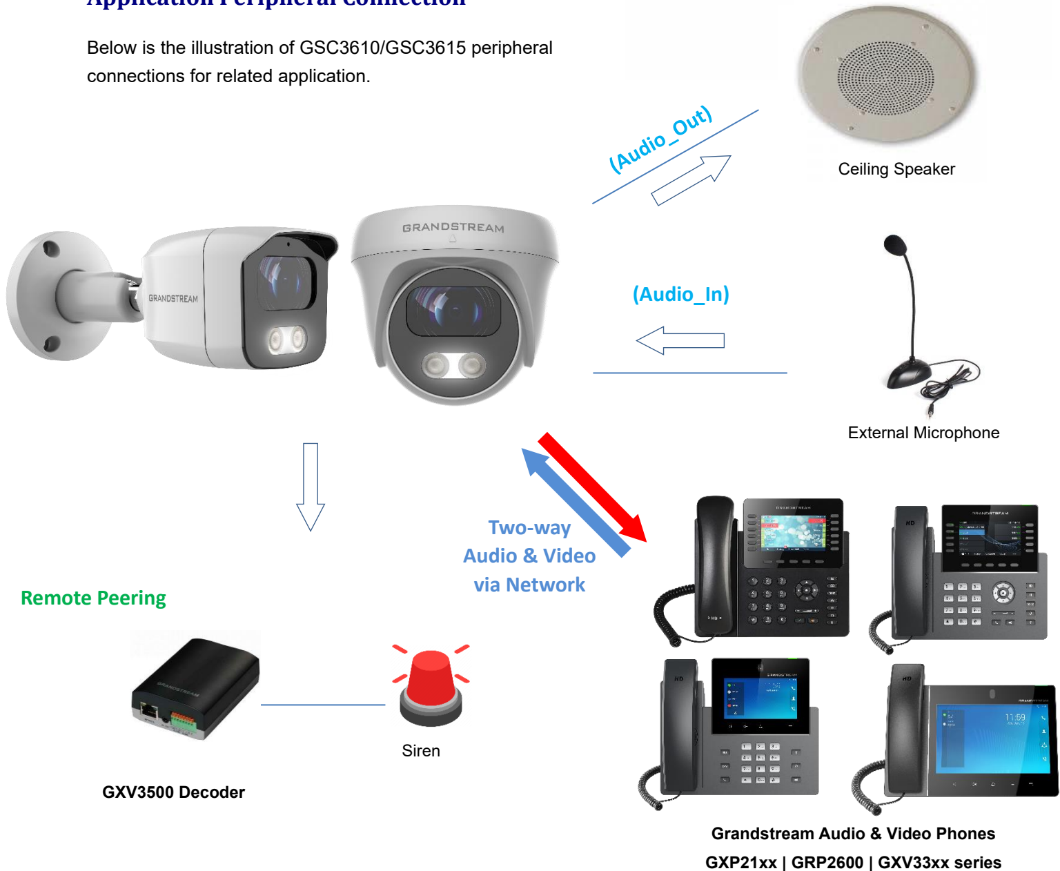
Figure 7: Application Peripheral Connection for GSC3610/GSC3615
