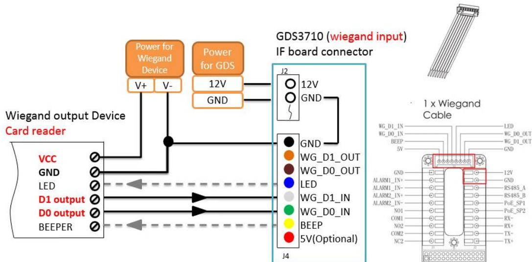
Figure 26: Wiegand Input Example with 3<sup>rd</sup> party Power Supply
