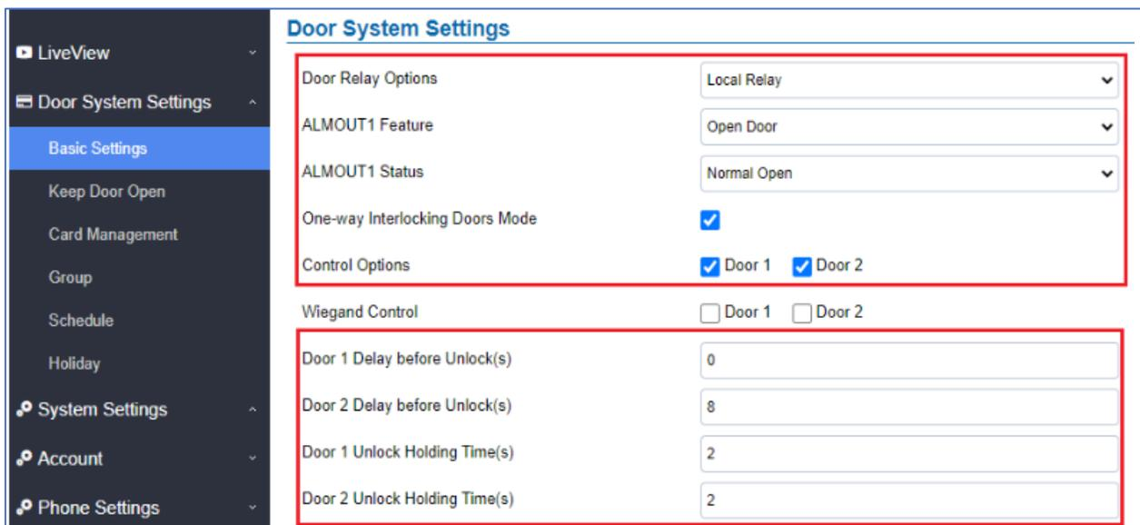
Figure 40: One-Way Interlocking Mode\_GDS3710\_Configuration\_1
