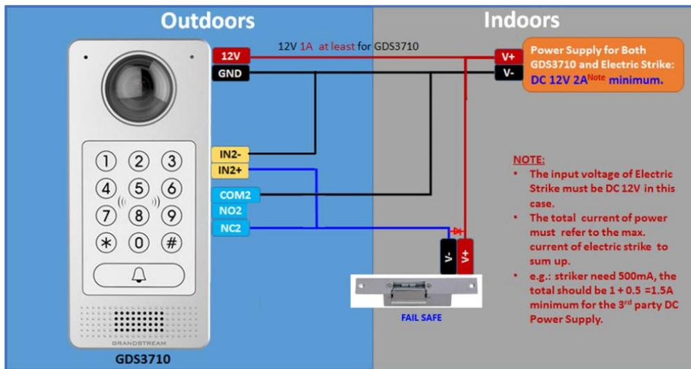
Figure 31: “Fail safe” Electric Strike using 3<sup>rd</sup> Party Power Supply
