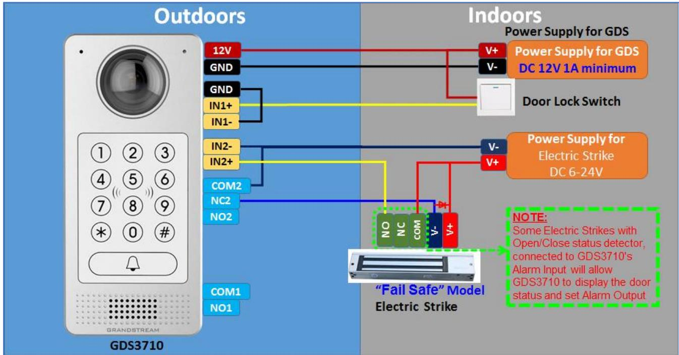
Figure 21: 3<sup>rd</sup> party Power Supply Wiring Sample
