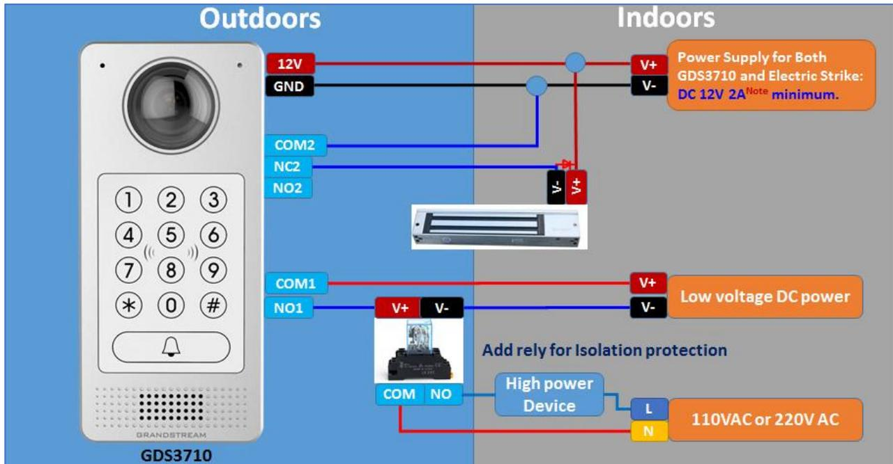
Figure 25: Electric Strike and High-Power Device Example
