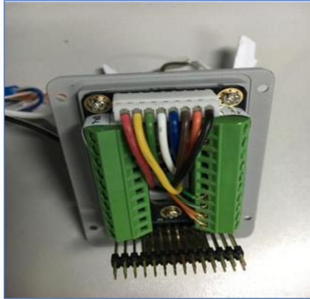
Figure 115: Wiegand Interface Cable
