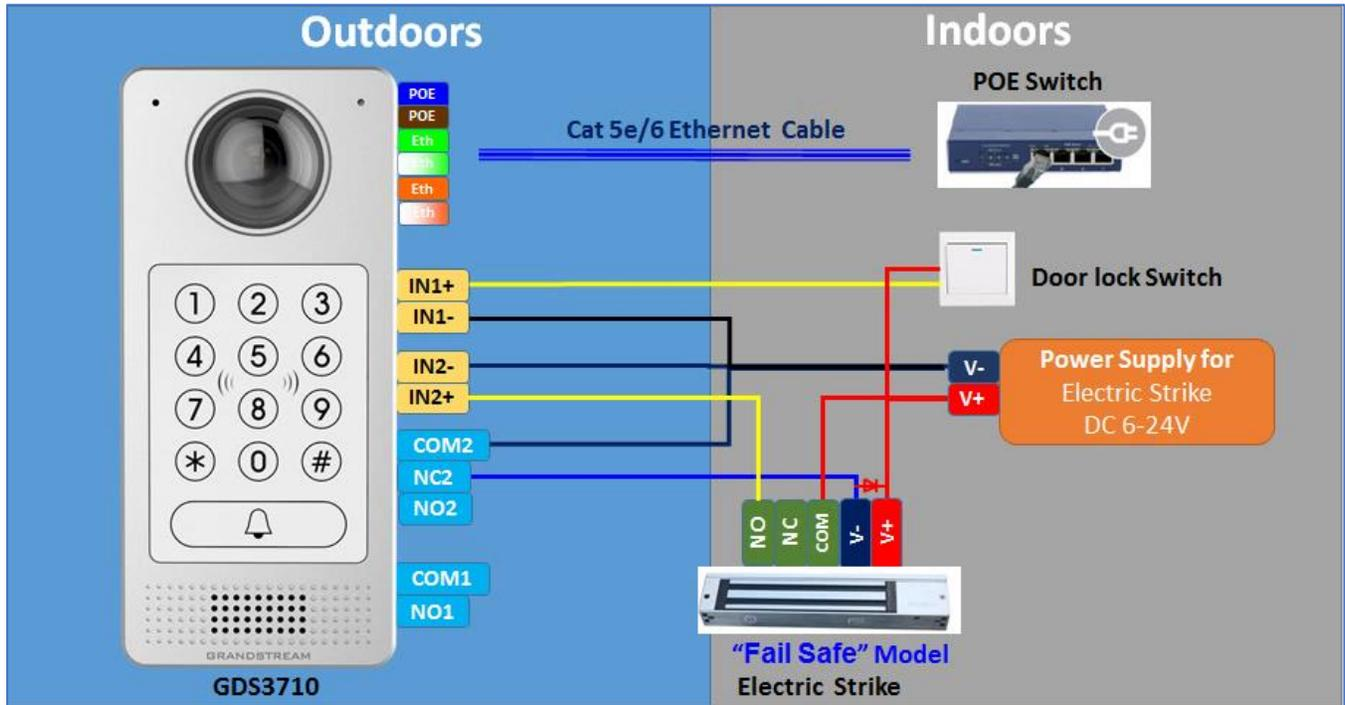
Figure 23: Wiring Sample using PoE to power GDS3710 and 3<sup>rd</sup> party Power Supply for Electric Strike
