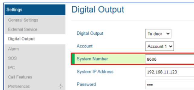
Figure 38: GSC3570 secure open door via GDS3710-GSC3570 Digital Input configuration
