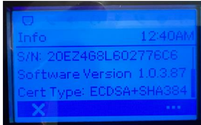
Figure 4: Certificate Type Display on GRP260X LCD
