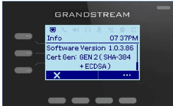
**Figure 4: Gen 2 Certificate Status on GRP260X LCD**
