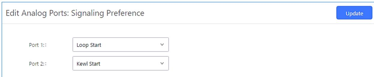
**Figure 102: FXS Ports Signaling Preference**
