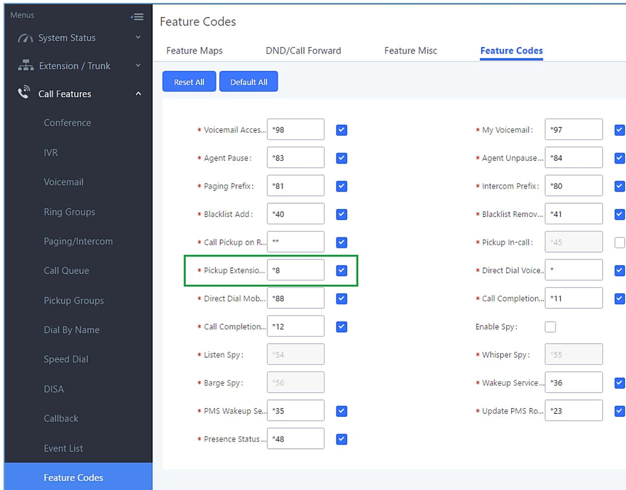
The screenshot shows the 'Feature Codes' configuration page in the Grandstream web interface. The left sidebar contains a 'Menus' section with 'Call Features' expanded. The main content area is titled 'Feature Codes' and has tabs for 'Feature Maps', 'DND/Call Forward', 'Feature Misc', and 'Feature Codes'. Below the tabs are 'Reset All' and 'Default All' buttons. The configuration table lists various feature codes with their corresponding values and checkboxes.
