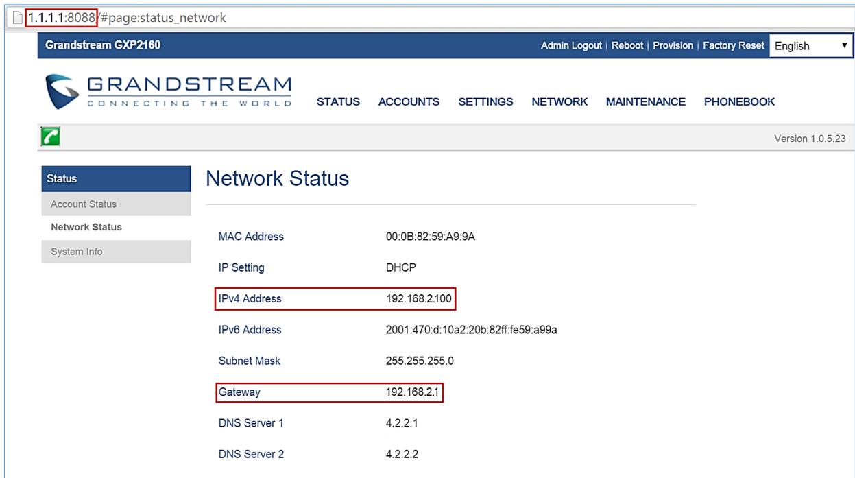
**Figure 21: GXP2160 Web Access Using UCM6510 Port Forwarding**
