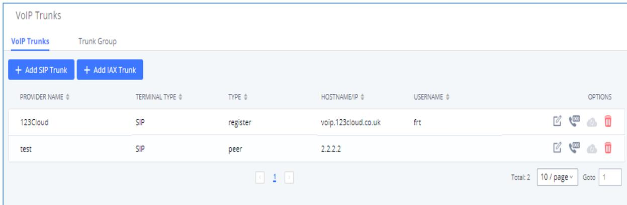
The screenshot shows the 'VoIP Trunks' management page. It includes two buttons: '+ Add SIP Trunk' and '+ Add IAX Trunk'. Below is a table with columns: PROVIDER NAME, TERMINAL TYPE, TYPE, HOSTNAME/IP, USERNAME, and OPTIONS. Two trunks are listed: '123Cloud' (SIP, register, voip.123cloud.co.uk, frt) and 'test' (SIP, peer, 2.2.2.2). The page also shows pagination controls: Total: 2, 10 / page, and Goto 1.
