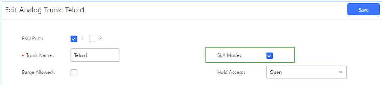
**Figure 116: Enable SLA Mode for Analog Trunk**
