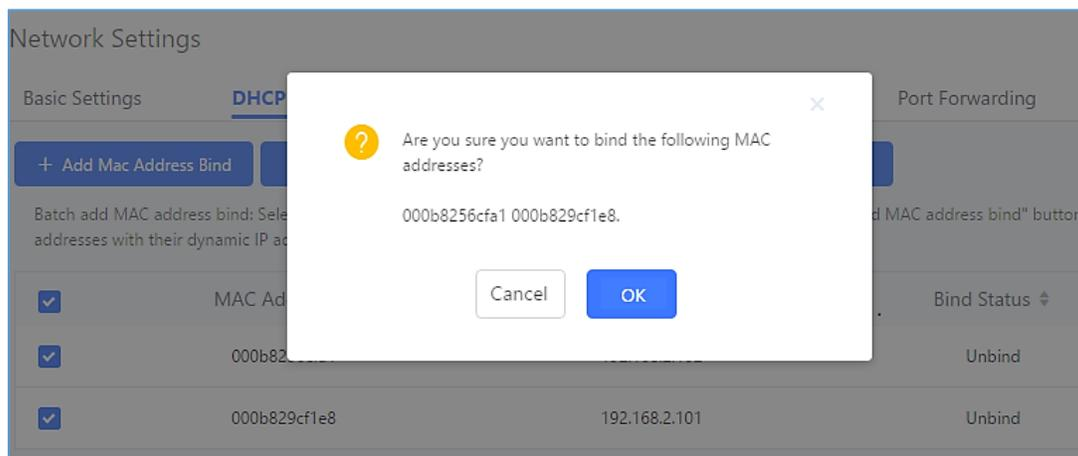
**Figure 14: Batch Add MAC Address Bind**
