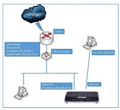
Figure 12: UCM6202 Network Interface Method: Switch
