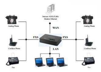
Figure 3: Connecting the HT818
