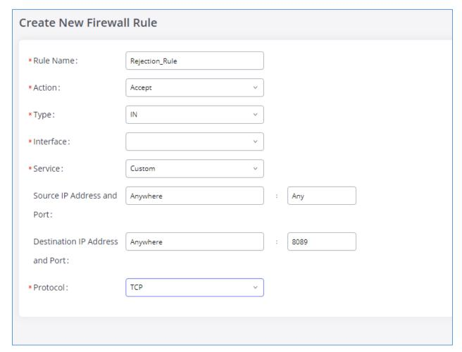
Figure 28: Create New Firewall Rule
