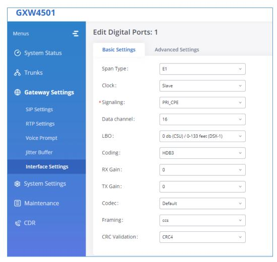
Figure 46: Digital Port Configuration
