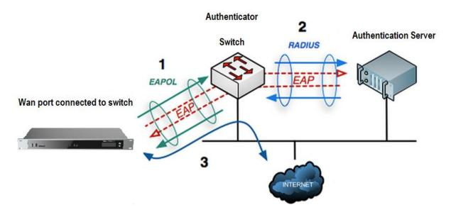
Figure 22: GXW450X Using 802.1X as Client
