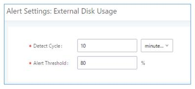
Figure 72: System Events → Alert Events Lists: External Disk Usage
