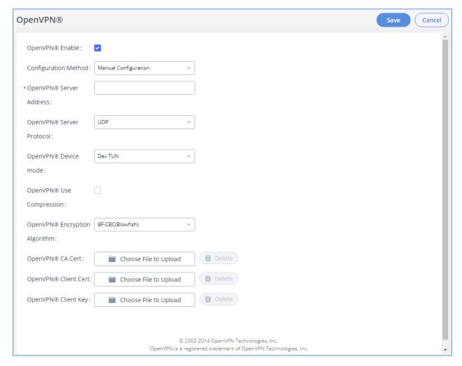
Figure 24: OpenVPN® Feature on the GXW450X
