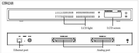
Figure 1: Diagram of GXW4216/24/32/48 Panel
