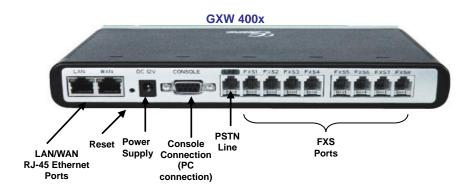
Figure 1: Diagram of GXW4004-8 back panel
