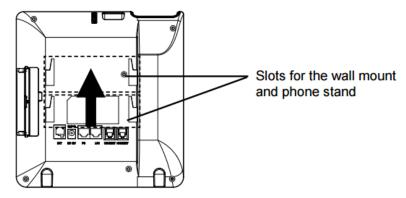
Figure 2: Slots For The Wall Mount And Phone Stand On The GXV3240.
