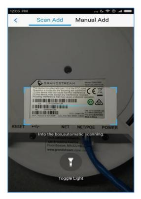
Figure 7 : Adding New AP by Scanning the Barcode
