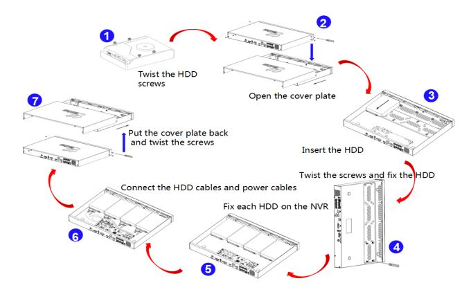
Figure 1: GVR3550 HDD Installation
