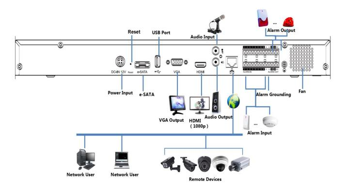
Figure 2: GVR3550 System Connection Diagram
