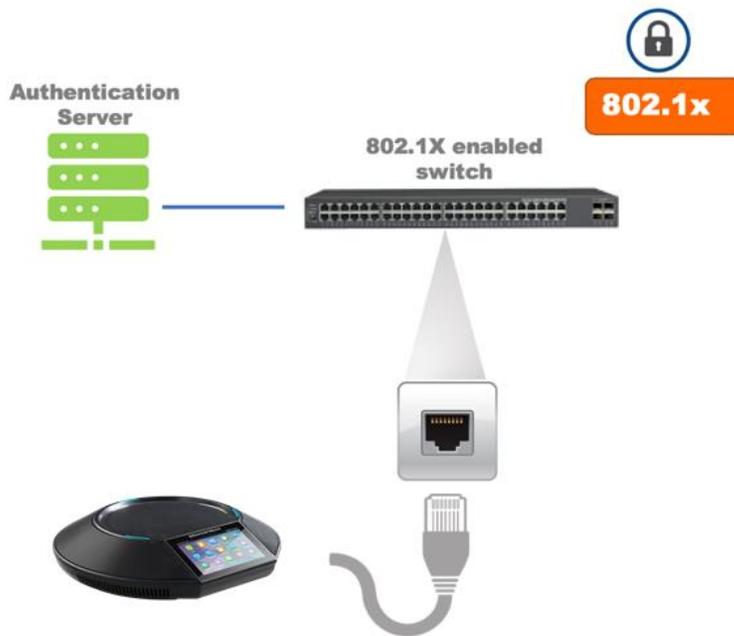
**Figure 15: 802.1X for GAC2500 Deployment**
