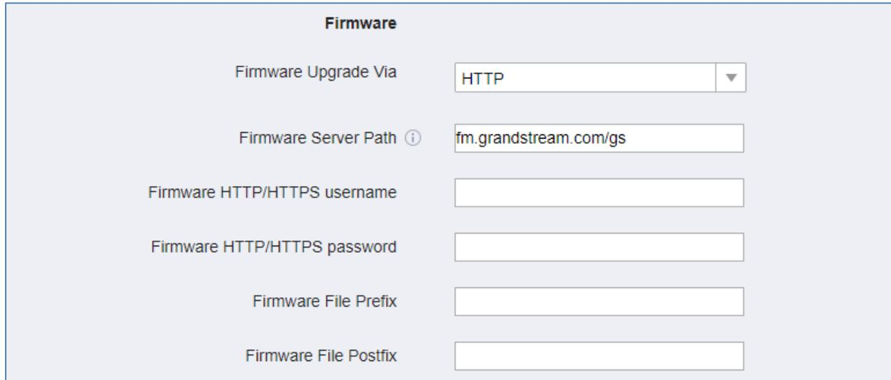
Figure 19: GAC2500 Firmware Upgrade Configuration
