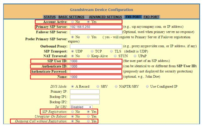
Figure 4: Configure FXS Port on the HT503
