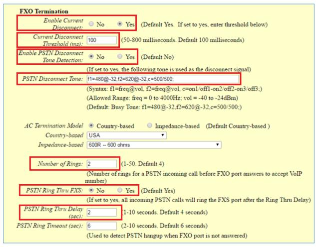
Figure 16: Configure FXO Port on the HT503: FXO Termination
