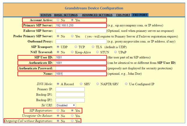
Figure 5: Configure FXO Port on the HT503 - Registration
