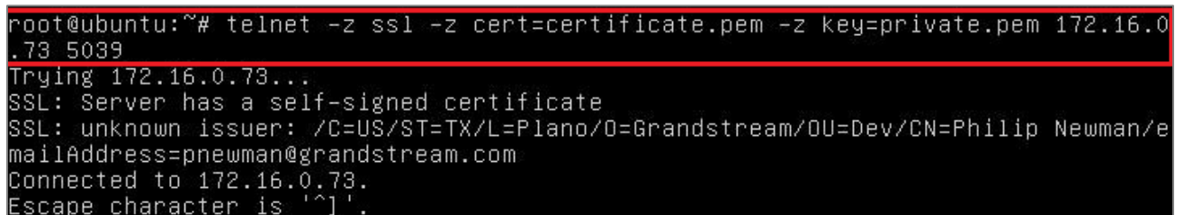
Figure 9: Telnet Connection to AMI Using TLS
