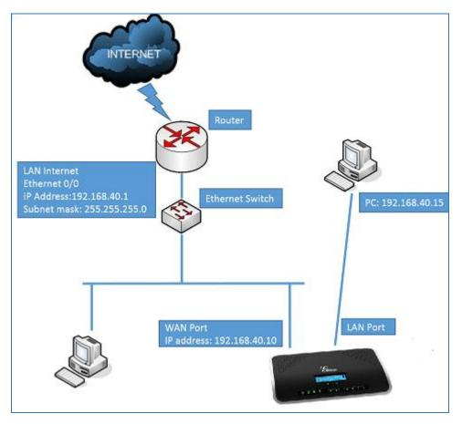
Figure 24: UCM6102 Network Interface Method: Switch
