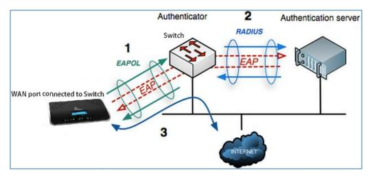
Figure 26: UCM6100 Using 802.1X as Client
