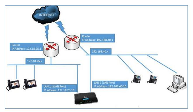
Figure 25: UCM6102 Network Interface Method: Dual
