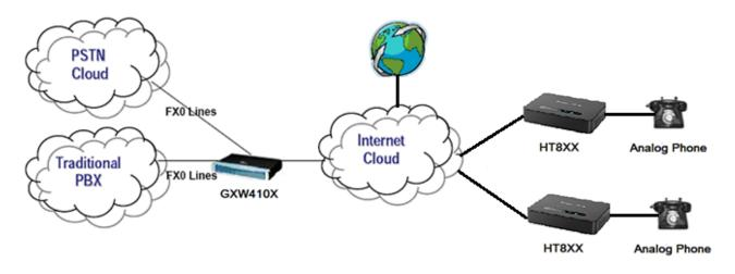
Figure 2 : Scenario 2: Peering multiple HT8XX with GXW410X
