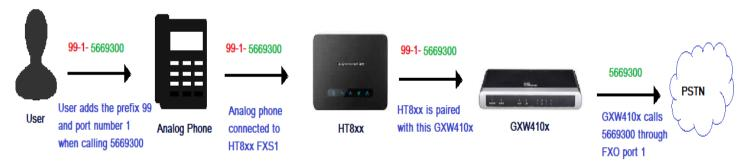
Figure 14: One-To-One Mapping
