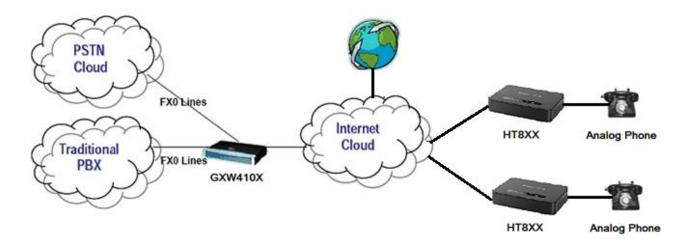
Figure 16: Peering Multiple HT8XX with GXW410X
