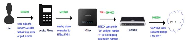
Figure 15: Port-To-Port Mapping call flow
