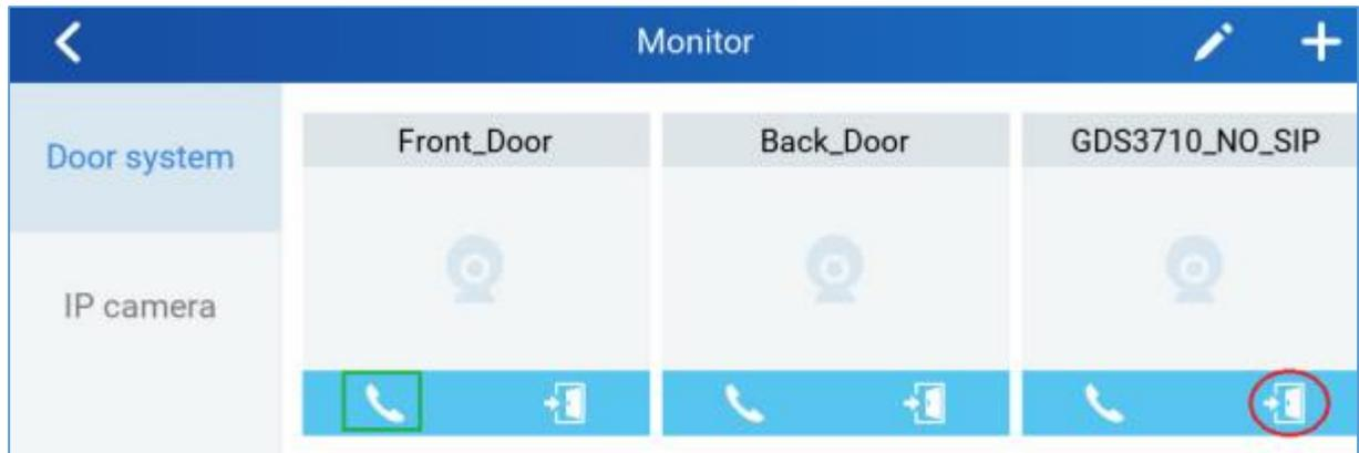
**Figure 9: GSC3570 LCD screen - Door system**
