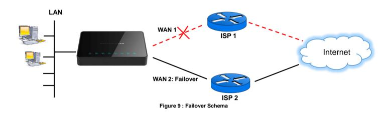
The advantage of failover in this case is to ensure that all traffic is going through a single path, which is helpful for path-sensitive connections such as VPN traffic. But the disadvantage is the bandwidth of the backup connection being unused, which is not the case for Load Balancing using the bandwidth of both Internet connections.
