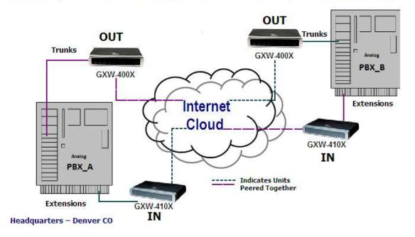
Note: For each direction, you can have X simultaneous calls per X amount of ports connected from PBX to each gateway. For example If connecting all ports then: with GXW4x04 you can have up to 4 simultaneous calls, with GXW4x08 you can have up to 8 simultaneous calls.
