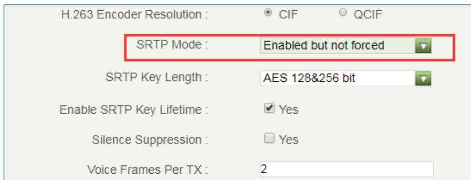
**Figure 10: Configure SRTP Mode on Clients**
