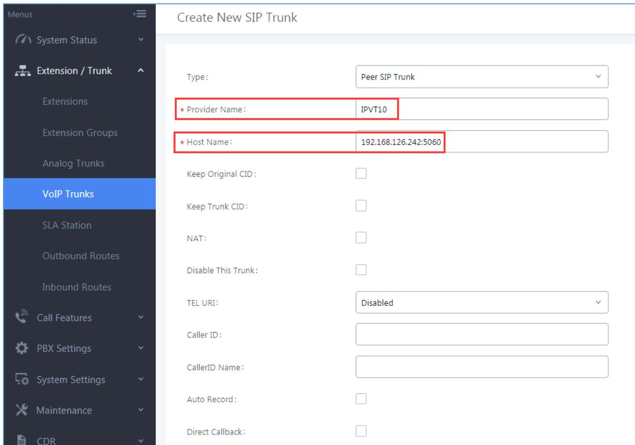
**Figure 2: Configure VoIP Trunk**
