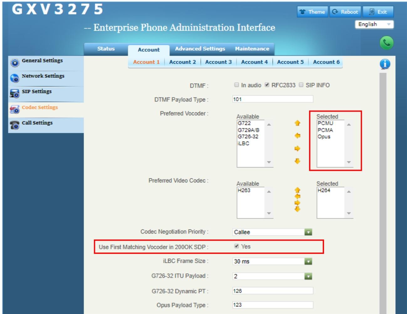
**Figure 9: Configure Codecs on Clients**
