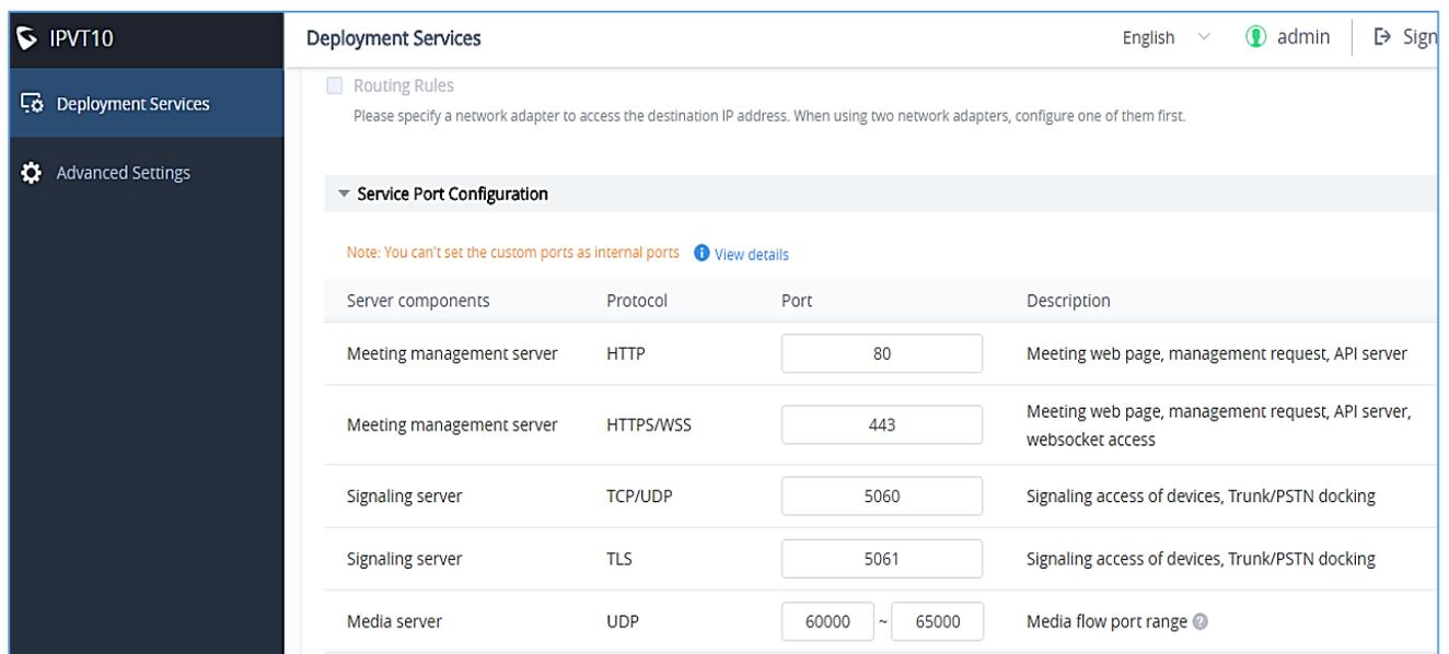
The screenshot shows the 'Deployment Services' configuration page in the IPVT10 Web Management UI. The 'Service Port Configuration' section is expanded, displaying a table with the following data:
