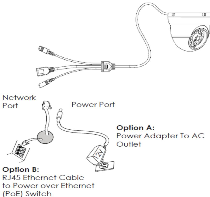
**NOTE:** Choose Option A if using the power supply; or choose Option B if using a Power over Ethernet (PoE) switch.
