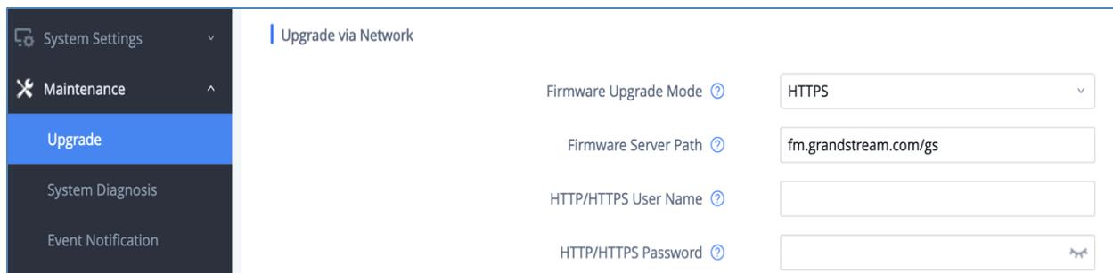
Figure 24: GXV33XX Firmware Upgrade Configuration
