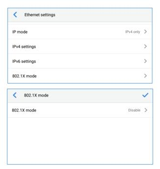
Figure 6: 802.1X Keypad Menu Configuration
