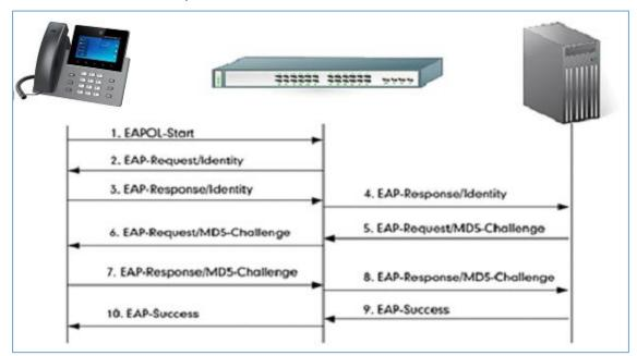
Figure 12: 802.1x Authentication Using MD5
