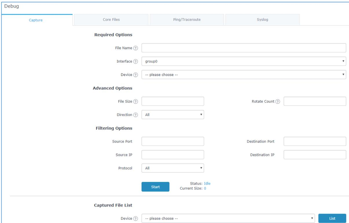
The screenshot shows the 'Debug' menu with 'Capture' selected. It features three tabs: 'Core Files', 'Ping/Traceroute', and 'Syslog'. The 'Capture' tab is active and contains the following sections:
