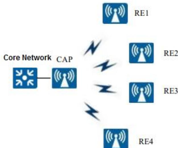
Figure 3: Mesh Network - Star Mode
