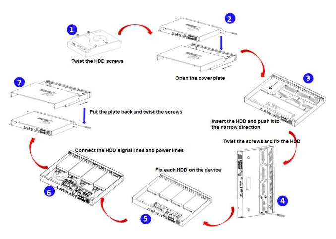
Figure 5 GVR3550 HDD Installation Diagram
