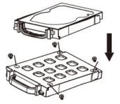
4. Push the HDD case into the slot in upright position until "click" sound heard;
