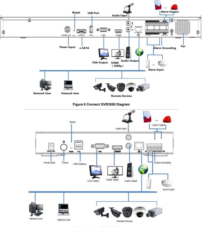
Figure 7 Connect GVR3552 Diagram
