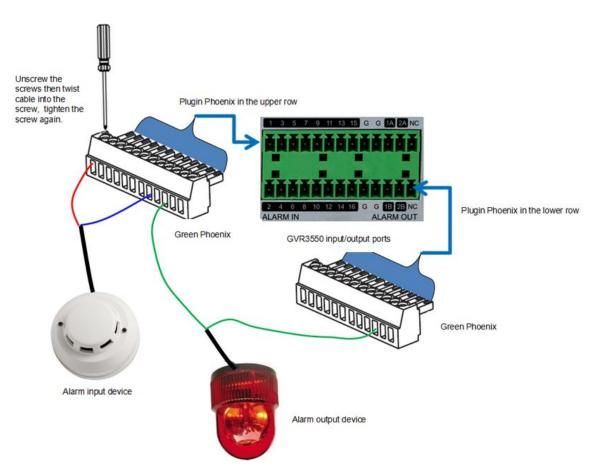
Figure 9 Alarm Device Connection Diagram
