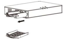
3. Put the 2.5" HDD into the HDD case in upright position then tighten the screws to install the HDD;
