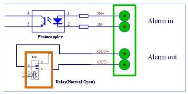
Figure 7: Alarm\_In/Out Circuit for GDS3710
