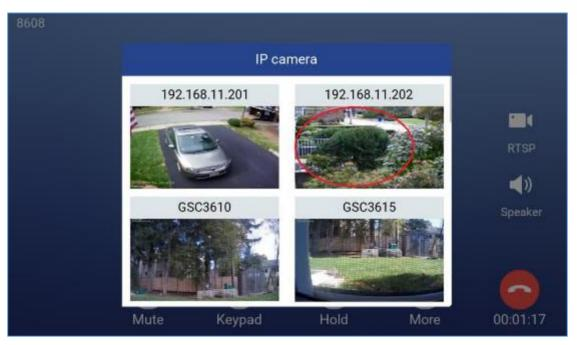
Figure 38: GSC3570 – Selecting RTSP video stream for IP camera
