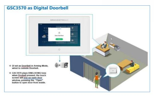
Figure 17: GSC3570 as Digital Doorbell and door opener example
