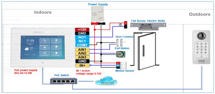
Figure 8: Fail Secure" Electric Strike, POE Power Supply
