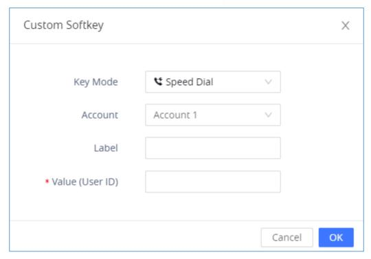
Figure 19: Add Custom Softkey in Idle Screen
