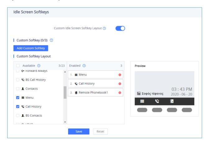
Figure 18:Idle screen softkeys settings customization
