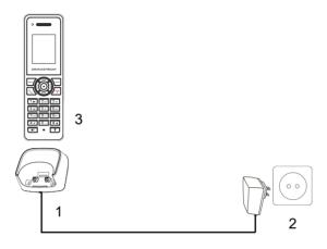
Figure 6: Setting up the charge station
