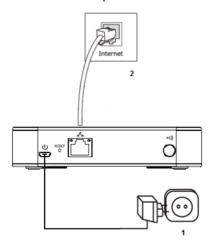
Figure 4: Connecting the Base station
