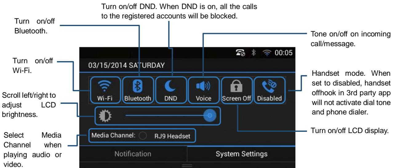
Figure 23: System Settings in Status Bar
