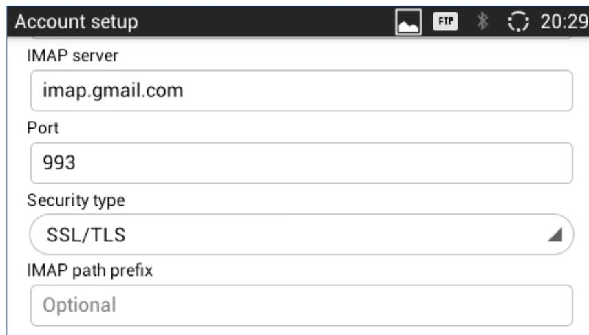
A screenshot of a mobile application's 'Account setup' screen for IMAP. The screen has a dark header with the title 'Account setup' and system icons (signal, FTP, Bluetooth, refresh, and time 20:29). Below the header are four input fields: 'IMAP server' with 'imap.gmail.com', 'Port' with '993', 'Security type' with a dropdown menu showing 'SSL/TLS', and 'IMAP path prefix' with 'Optional'.
